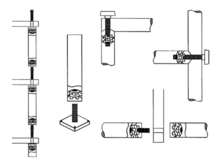
Inside Tube Diameter = 16,4-17,7Outer tube diameter = 3/4" Thread = M6
